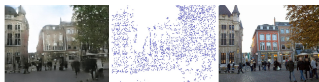
Figure 1: Reconstructed image (left) from extracted features (middle) closely resembles the ground truth (right).
