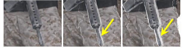
Figure 4: Ground truth and reprojection artifacts with translational prediction error of 10 cm (middle) and 20 cm (right).
