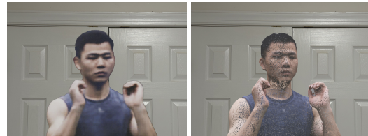
Figure 1: Comparison of volumetric content rendered on HoloLens, with NeRF (left) and point cloud (right).
